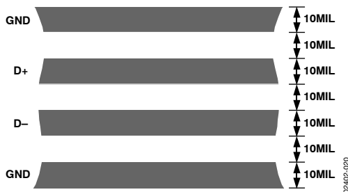
Figure 20. Arrangement of Signal Tracks
